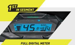
Always stay up-to-date with the Full Digital Meter which displays Real-time Fuel-efficiency, Average Fuel-efficiency, Distance-to-empty, Service Due Indicator, Gear Position Indicator & Eco Indicator.
